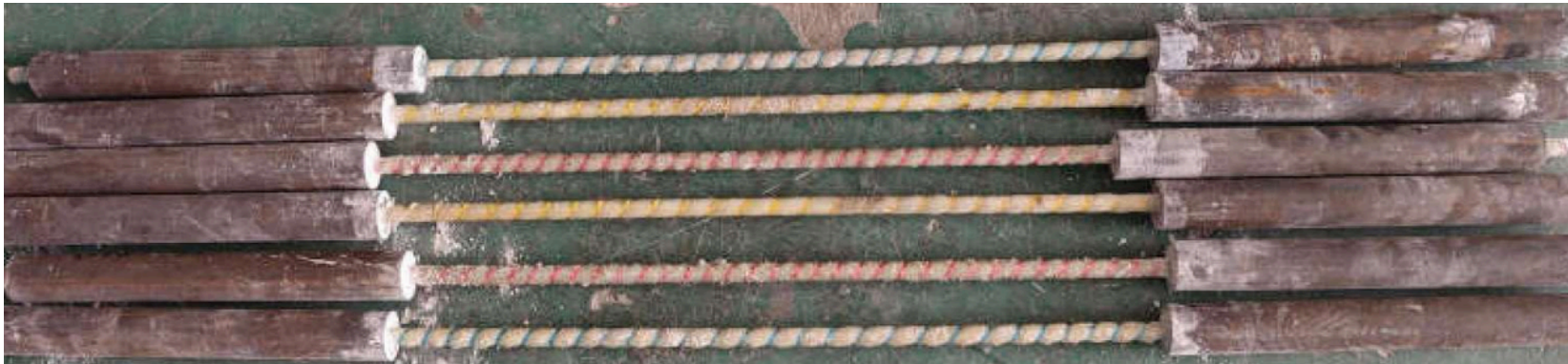
Rebar specimen length: 1000mmAnchor length: 250mm
