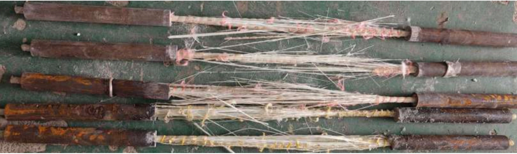
Representative failure mode of tensile test
