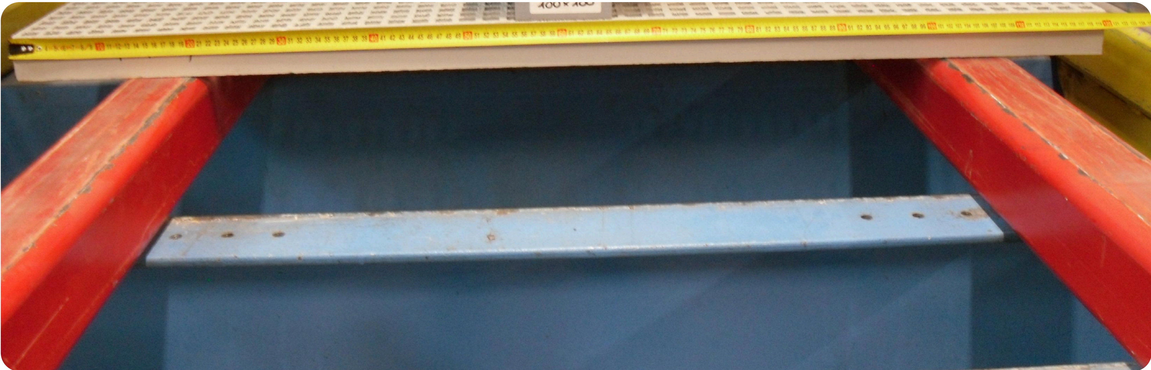
Front view showing load block, tape measurement, and supported panel span
