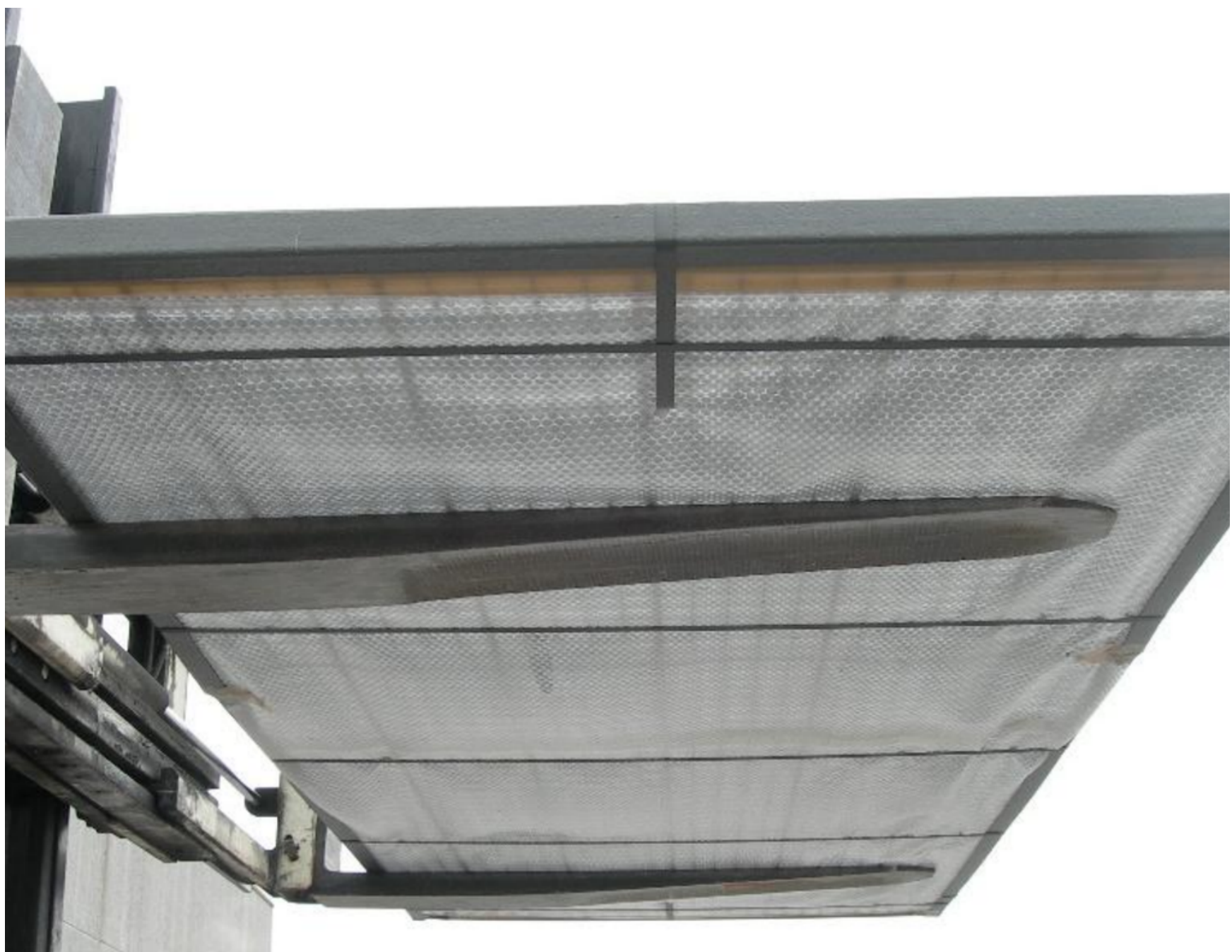
Forklift-supported handling of a wrapped grating bundle
