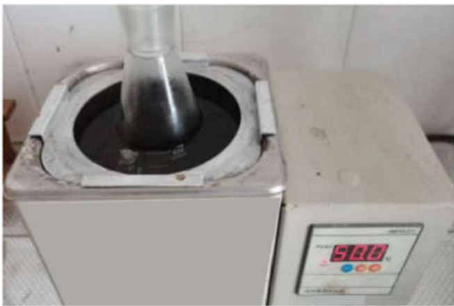
Maintaining uniform temperature of water at 50°C ±3°C for 24 hours
