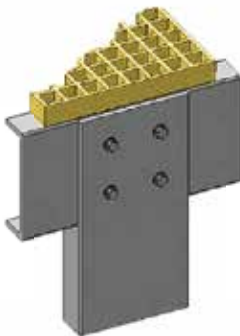
PFC COLUMN CONNECTION (FLANGES INWARD)
